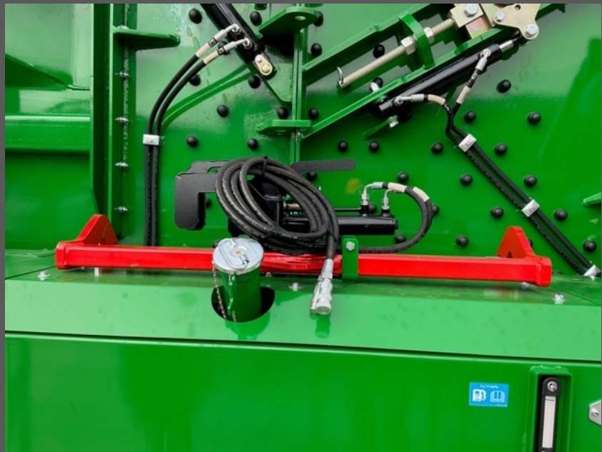
➤ Extraction tool for changing blow bars
