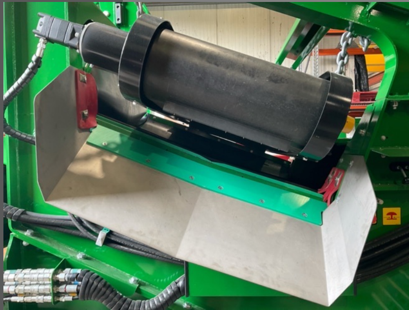
➤ Twin pole magnet for discharge chute
