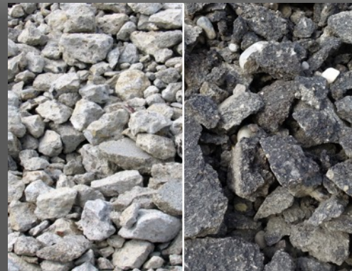
➤ Concrete & Asphalt Recycling
