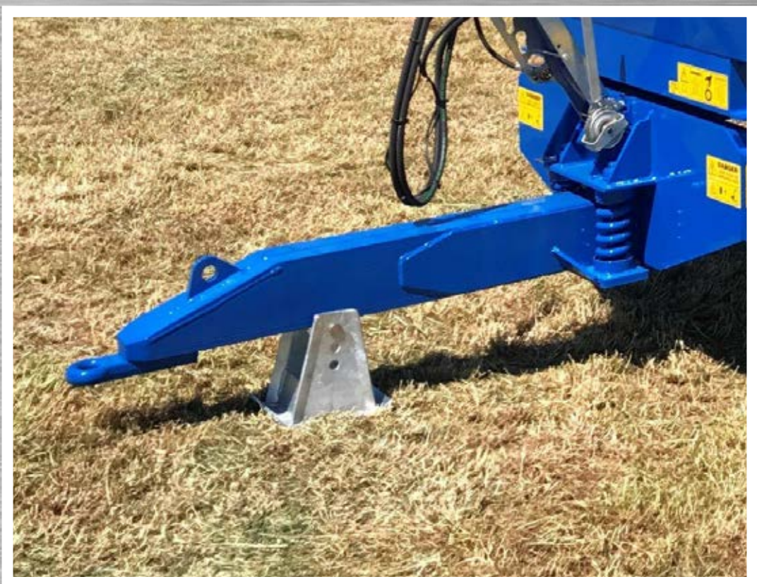
Sprung Drawbar Complete with Galvanised Parking Stand
